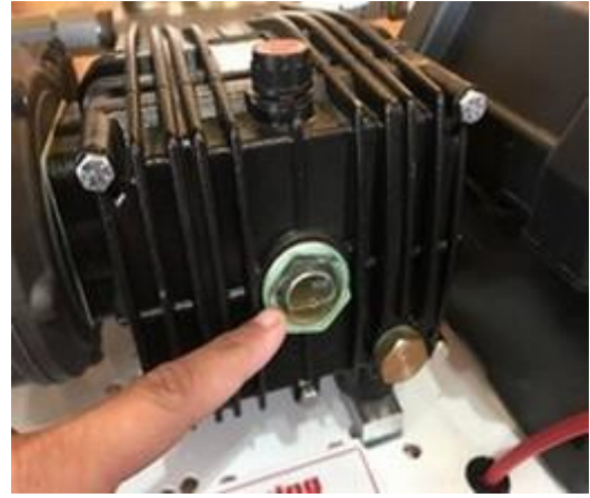
Figure #2 – Oil Level in Pressure Pump
