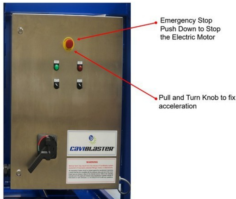
Figure 5.1 –Emergency Shut Down Switch On
