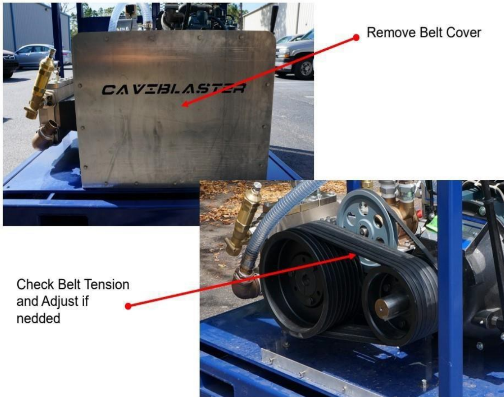
Figure 6.2 – Belt Inspection / Tension
