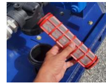
Check filter. Clean if necessary
