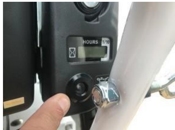
Figure #24 – Low Oil Level Warning
