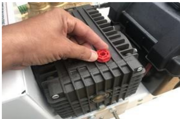
Figure #5 – Oil Filling Port in Pump
