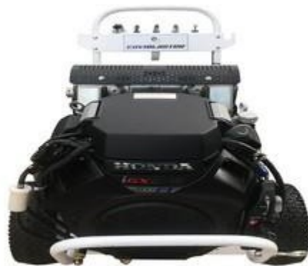
Figure #31 – Air Filter on Top of Engine
