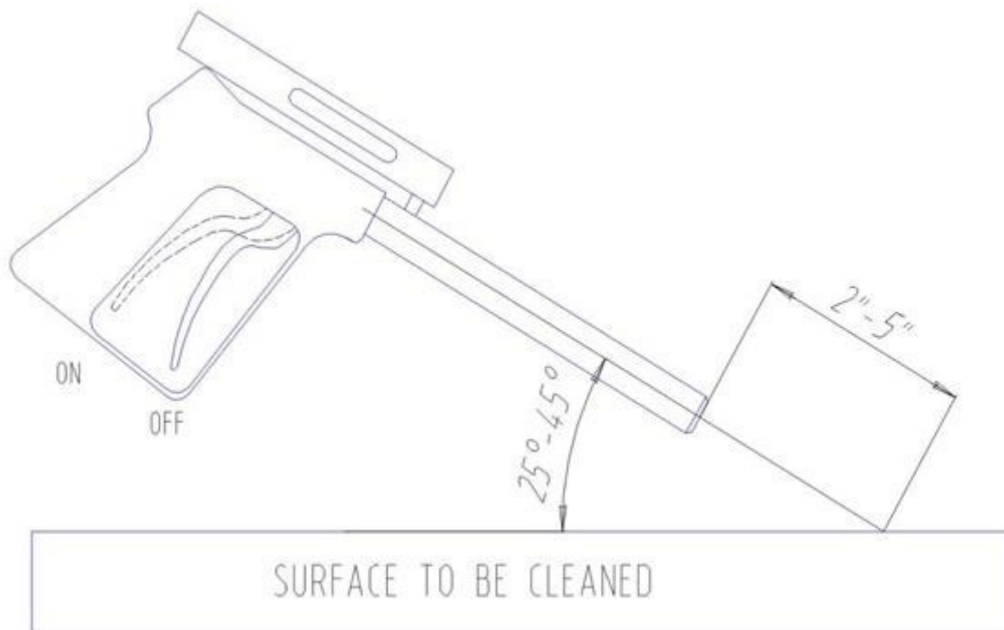
Figure 5.3 – Zero-Thrust Gun Position for Best Results
