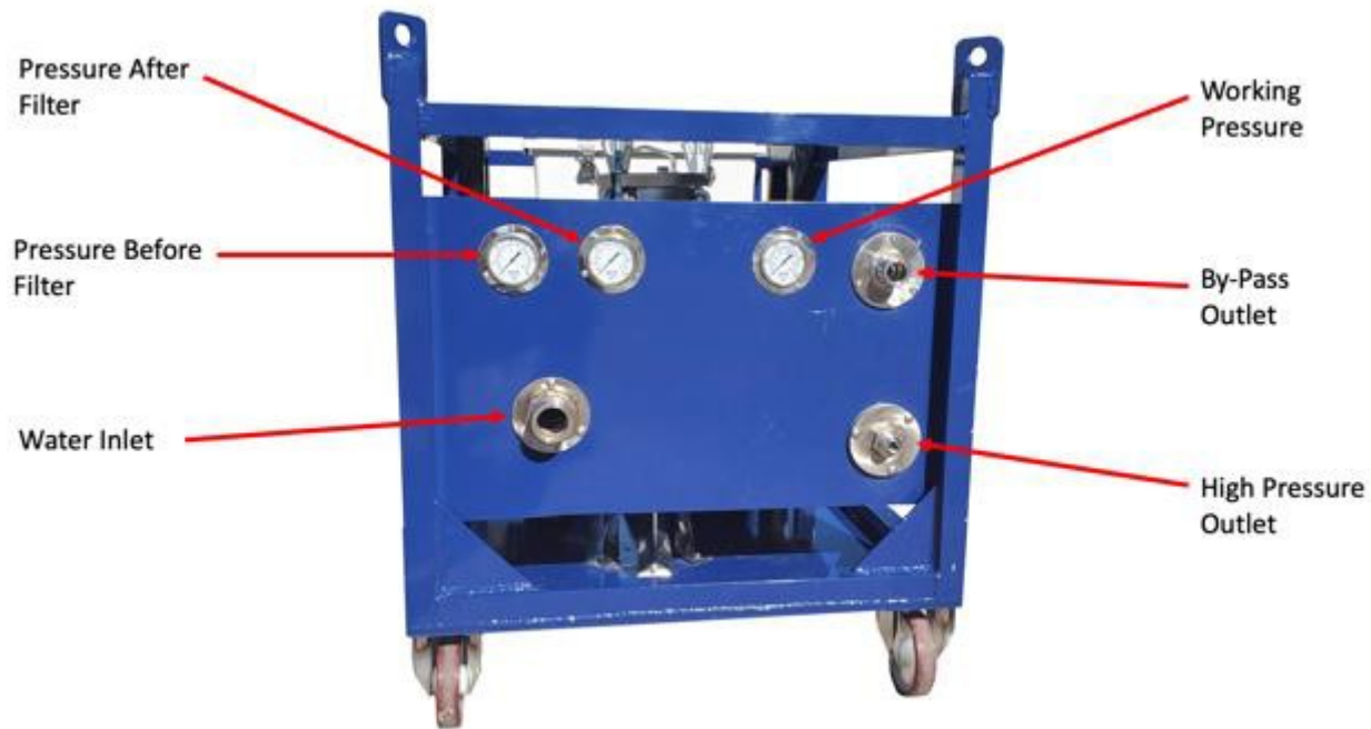
Figure 2.2 – CaviBlaster 1725-E Control Panel
