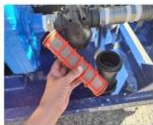
Check and Clean Strainer If Necessary
