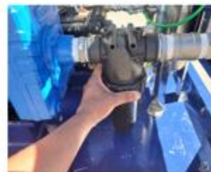
Screw tight to avoid leaks
