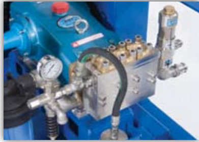
Stainless steel pump and appurtenances
