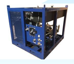
This unit is designed for cleaning with up to 3 Divers with ZT-Guns or 1 DoubleDome, great for cleaning FPSOs, LNGs, Tankers and Cruiser Liners, very big vessels by divers or with ROVs. Also preparing for SA 2.5 Inspections.
