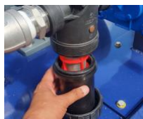
02-Pull case down to reveal filter
