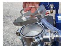
02-Pull lid up to reveal filter
