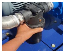
01-Unscrew the top and pull case down
