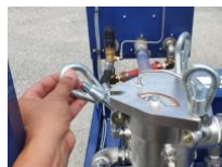
01-Unscrew and Remove 3 bow screws
