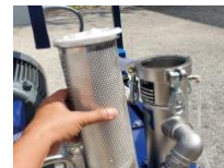
04-Place filter back in case and screw top lid again
