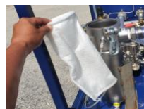
03-Check filter and change if necessary
