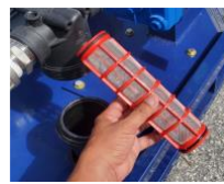
03-Check filter and clean if necessary
