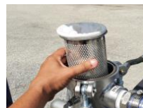
03-Check filter and change if necessary
