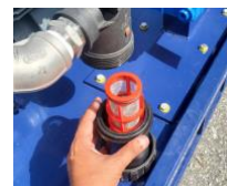
04-Place filter back in case and Push up and screw again
