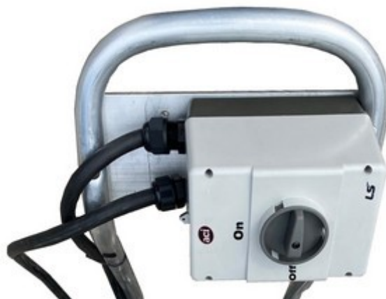
Figure #8 - Ignition Box
