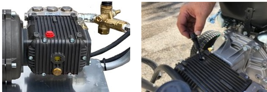
Figure # 2 - Pump Oil Level
