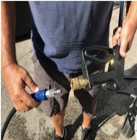
Figure #7 - Connecting the gun to the High Pressure Hose
