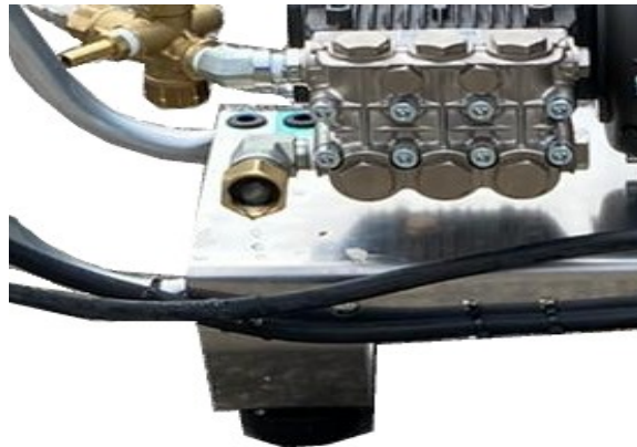
Figure #4 - Connect Garden Hose to Water Inlet
